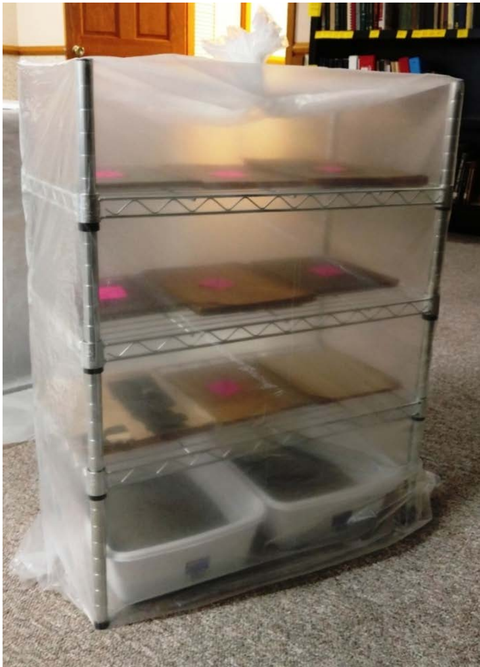
The combination of a chrome-plated wire baker's rack and a large plastic bag creates an enclosure that can treat several books at a time. Photo courtesy Kim Ray.
