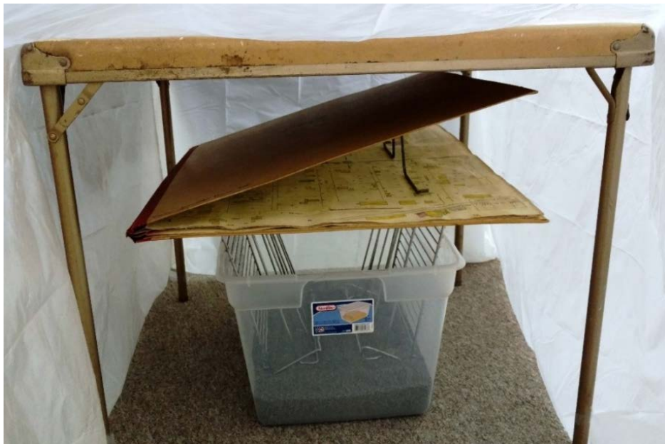
Treating oversized books requires an innovative approach. In this case, a card table provides the support necessary to create an enclosure using a large plastic sheet. Photo courtesy Kim Ray.
