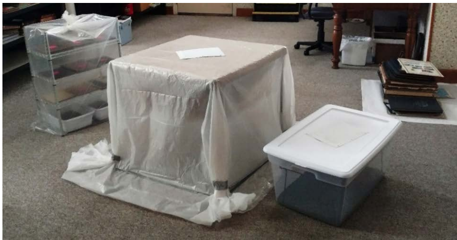
Air-tight enclosures in three unique configurations are made from readily available materials. Photo courtesy Kim Ray.
