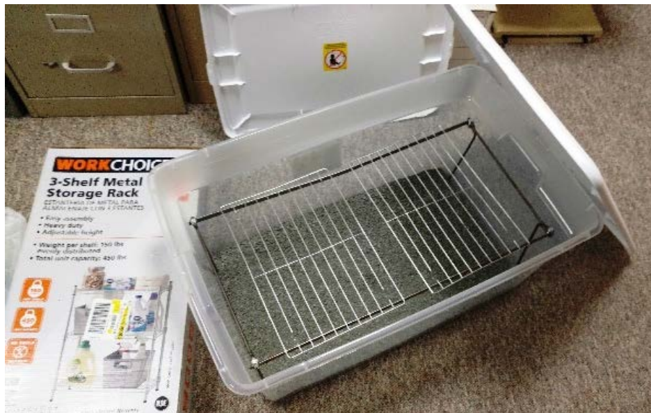
A plastic tote, a metal rack and unscented clay cat litter create a basic odor removal chamber. Photo courtesy Kim Ray.
